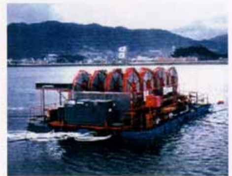
Pontoon for drain laying (4-stage 4-row simultaneous laying type)
